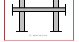
These two diagrams are a guideline to how the frame should be constructed but gusseting or triangulation is accepted.
